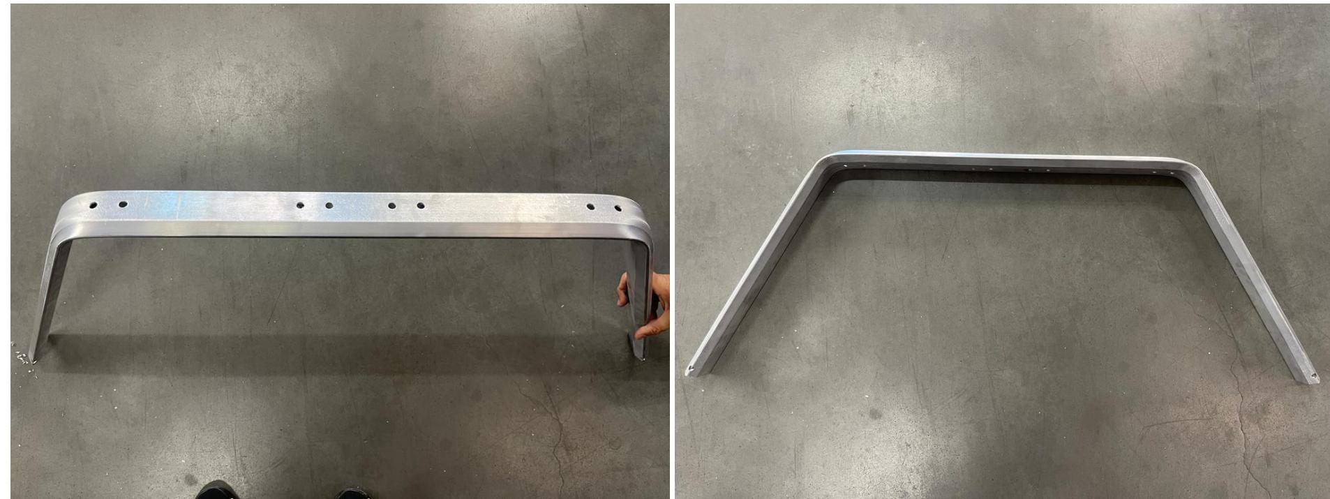
Bendind custom extrusion parts according to customer drawing.
