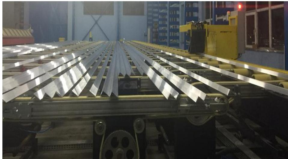
The aluminium billets are preheated to approximately  $480^{\circ}\text{C}$  and loaded in the 1660MT extrusion press. The machine pressed the billet in the container against the extrusion die forcing the aluminium billet to go through the die. The hot aluminium extrusion comes the out of the press exit platen.
