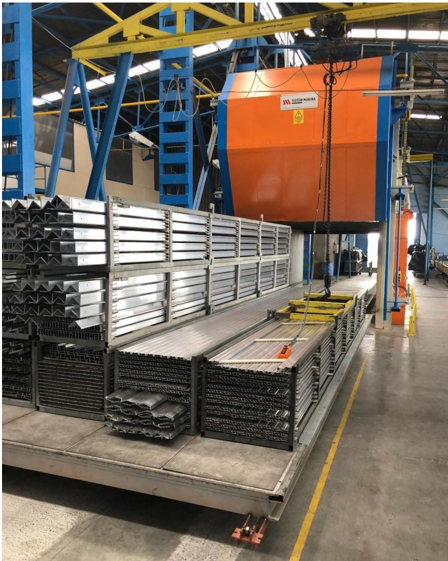
After the extrusion the profiles are in a soft state. In order to achieve mechanical properties the extrusion profiles are heat threaded in the aging oven.
