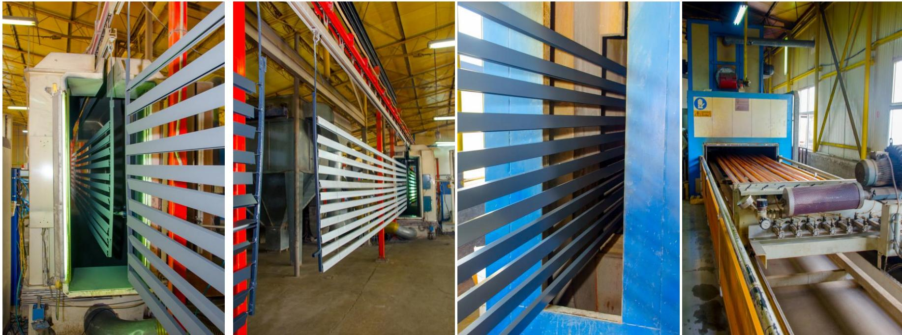
The powder coating of the profiles are done in the powder coating booth produced by Nordson by the automatic powder guns.
